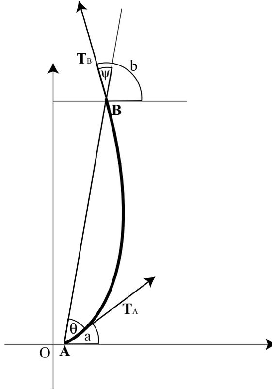
Figure 1: T-cubic spiral interpolating  $G^1$  Hermite data taken from a spiral.
