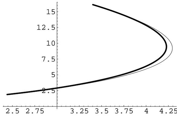
Figure 2: Quadratic spline approximation (thin mode) of spiral (thick mode) from (1).
