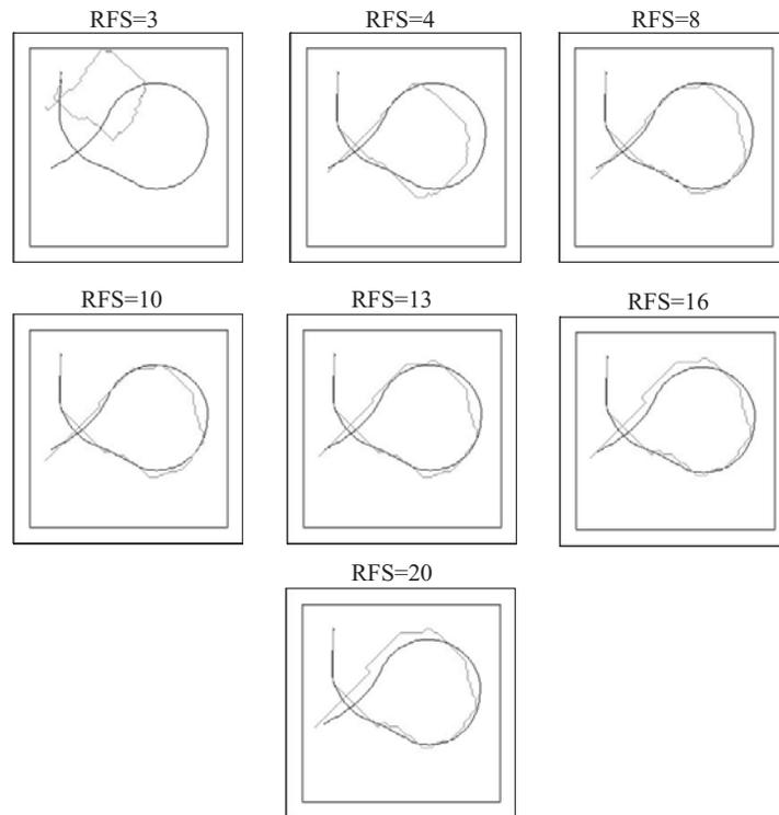
Figure 4: The effect of varying receptive field size with a fix RF distribution of 11664 cells. (RFS=Receptive Field Size expressed in pixels). The solid darker line shows the real trajectory of the object; the lightest shows the calculated trajectory using speed estimation and direction selectivity cells data.
