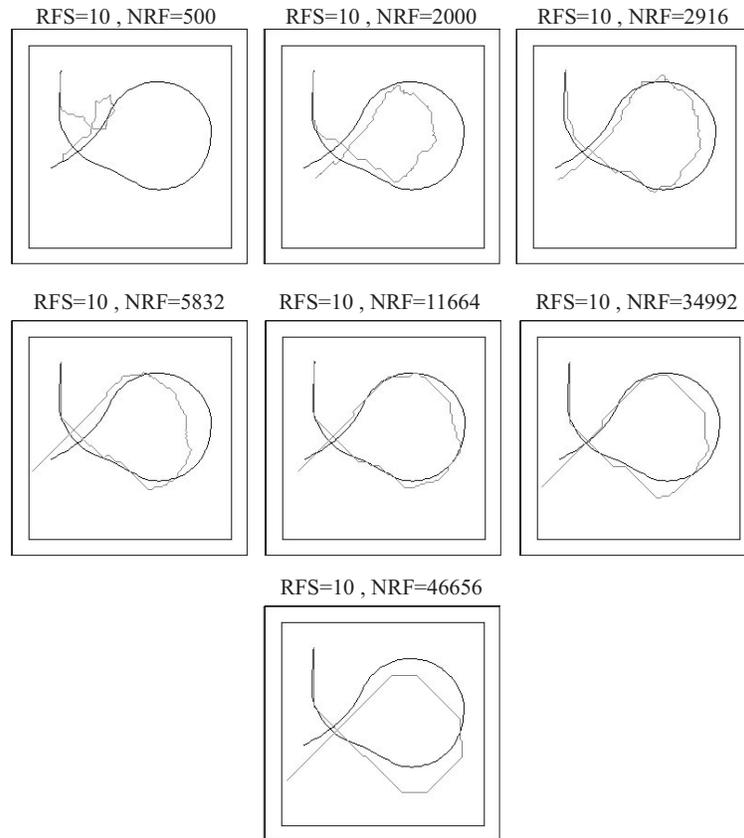
Figure 5: The effect of varying receptive field number with a fix RF size of 10 pixels. (NRF=Number of Receptive Fields randomly distributed over the input image). The solid darker line shows the real trajectory of the object; the lightest shows the calculated trajectory using data from speed estimation and direction selectivity cells.
