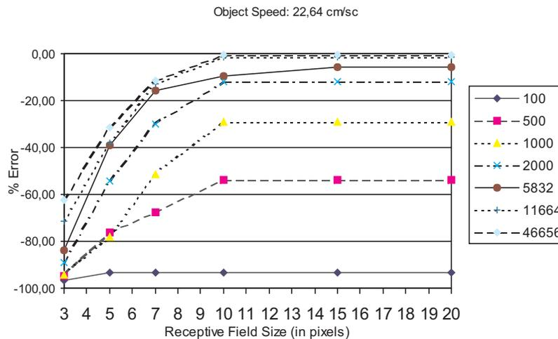
Figure 3: Percent error in the estimated speed vs. Receptive Field Size as function of the number of Receptive Fields.
